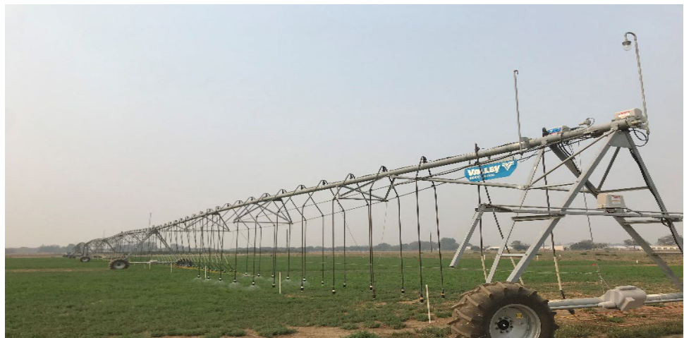
Figure 2. Linear Overhead Irrigation System was established in alfalfa at University of California Davis. Two systems (LESA and MDI) were compared in separate blocks with various deficit watering regimes.
